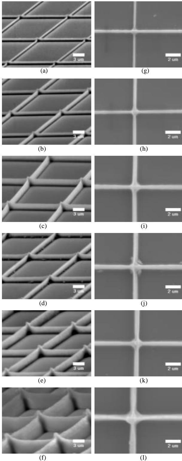
Figure 3. The SEM images of the micro-well structure made by TPA photopolymerization with single-line scanning method. Their pre-exposure time varies from 0 to 25 s in steps of 5 sec. (a) to (f) are taken from 75° tilt from normal direction and (g) to (l) are taken from the top of the samples.
