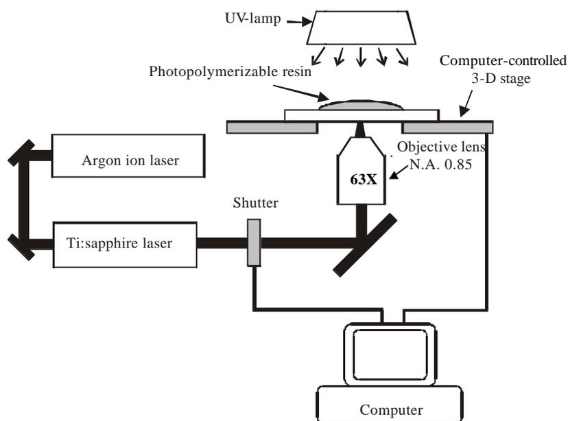
Figure 1. Schematic drawing of the experimental setup. A 4W UV-lamp is held at 3 inches above the samples to pre-cure the liquid resin.
