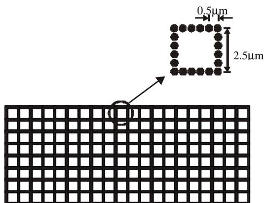
Figure 5. Layout of the micro-well structure for pinpoint scanning method.
