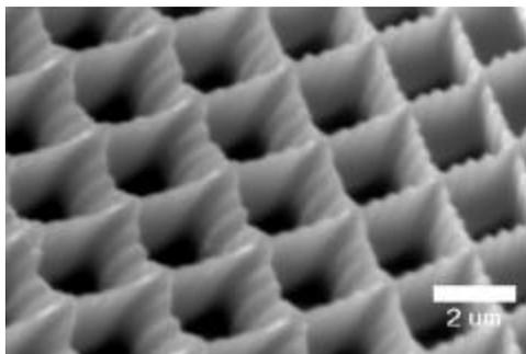
Figure 6. The SEM image of the micro-well structure made by pinpoint scanning method. Each point is exposed to IR laser pulse for 100 ms. (without UV pre-exposure)
