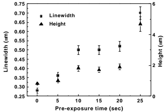
Figure 4. The measured linewidths and heights vs. UV pre-exposure time in samples made by raster scanning method.
