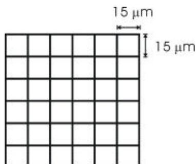
Figure 2. The micro-well pattern used for single-line scanning TPA photopolymerization.
