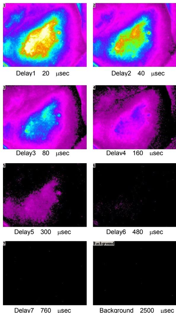
Figure 5. A demonstration of serial intensity images taken with the delay time sequence arranged specifically for Oxyphor R2. The ischemic area of the liver was prominent with the image taken after 300  $\mu\text{sec}$  delay time. The palette represented the 256 intensity levels (8 bits) digitized by the image processor board.
