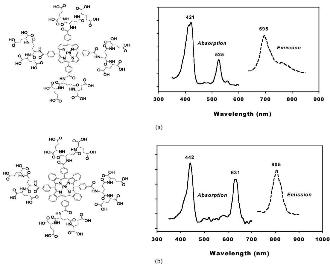
Figure 3. The chemical structure and absorption and emission spectra of (a) Pd-*meso*-tetra (4-carboxyphenyl) porphyrin-dendrimer (Oxyphor R2) and of (b) Pd-*meso*-tetra (4-carboxyphenyl) tetrabenzoporphyrin-dendrimer (Oxyphor G2).
