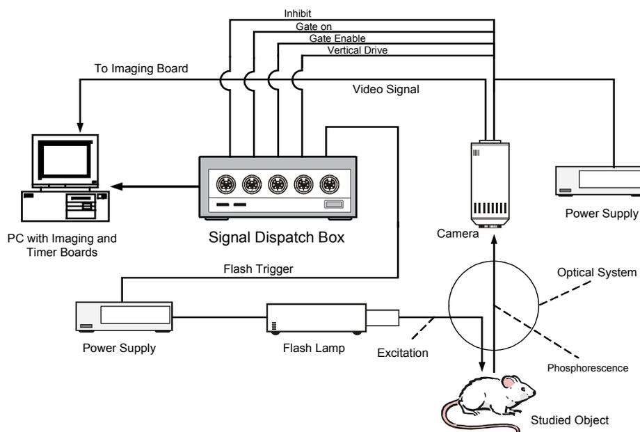
Figure 2. The schematic description of the oxygen imaging system.
