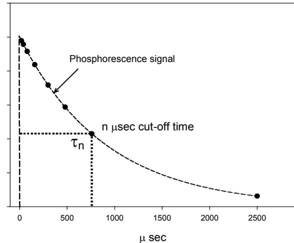
Figure 1. A typical phosphorescence single with single exponential decay. The delay time sequence which was set to acquire seven images, plus background image, for the phosphor Oxyphor R2 is: 20  $\mu$ sec, 40  $\mu$ sec, 80  $\mu$ sec, 160  $\mu$ sec, 300  $\mu$ sec, 480  $\mu$ sec, 760  $\mu$ sec, and 2500  $\mu$ sec.
