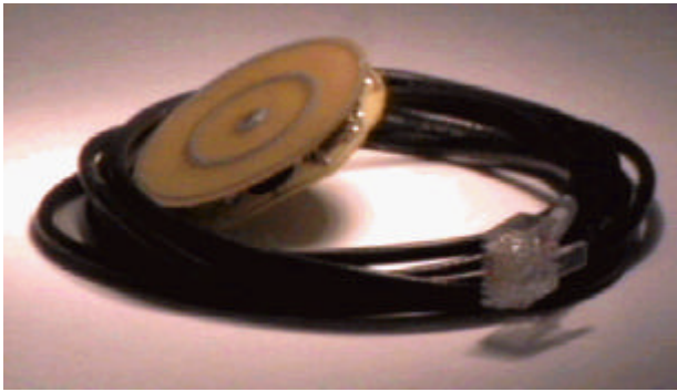
Figure 5 Finished active sensor with RJ-11 connector.
