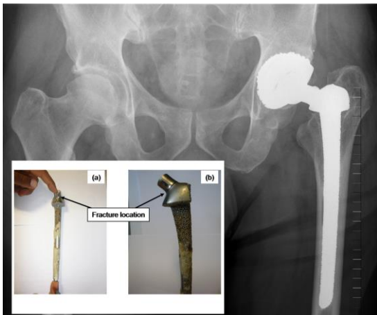
Figure 1. Anteroposterior radiograph showing prosthetic fracture at neck/stem transition. Insets (a) and (b) show the retrieved Lord femoral stem with a complete fracture at the neck/stem transition radius.
