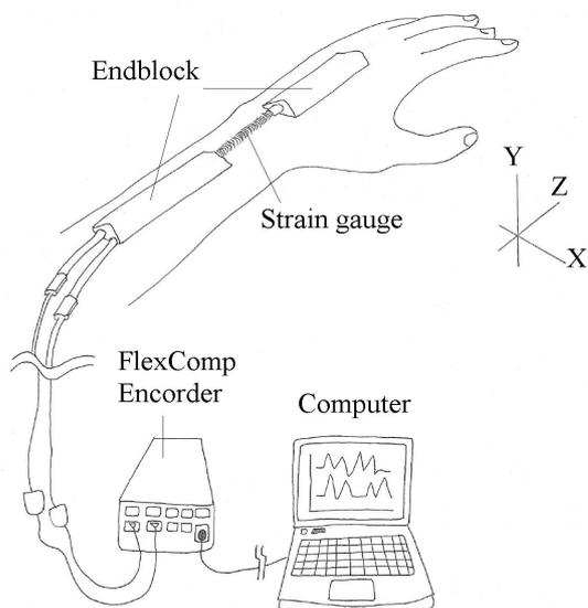
Figure 1. The experimental system and the coordinate system
