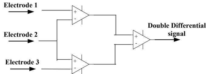
Figure 2. The architecture of double differential technique.
