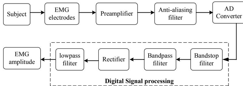
Figure 3. The EMG signal acquiring block diagram.
