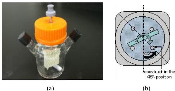
Figure 2. Spinner flask bioreactor is cell-culture system designed to enable the seeding and the growth of engineered tissues. (a) Dynamic seeding method with spinner flask (b) Top view of the bioreactor; the construct is at 45° position for maximum fibroblasts adhesion density.
