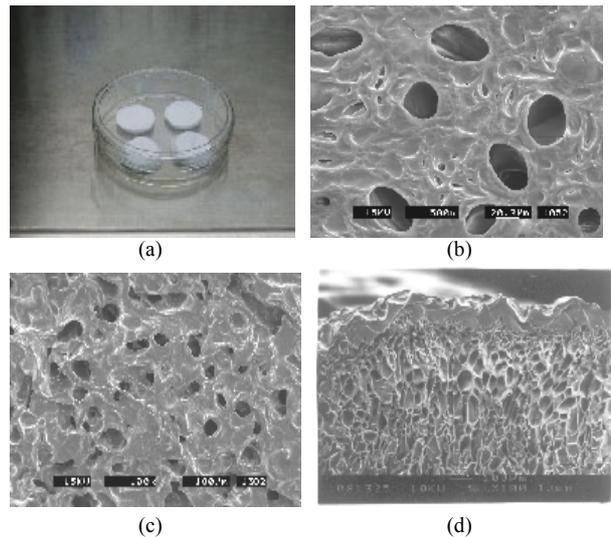
Figure 3. (a) The stereo appearance of fabricated gelatin-C6S-HA sponge. Scanning electron micrograph of gelatin-C6S-HA sponge freeze dried at  $-196\text{ }^\circ\text{C}$  (b) and  $-20\text{ }^\circ\text{C}$  (c), respectively. Rete ridges-like structure was indicated by the arrow shown in cross sectional view (d).
