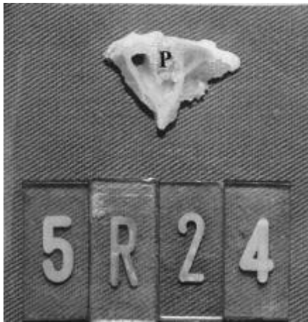
Figure 12. A piece of cross section of being grafted a composite of calcium sulfate and calcium phosphate at 24 weeks. The central part of implant has burst (P).
