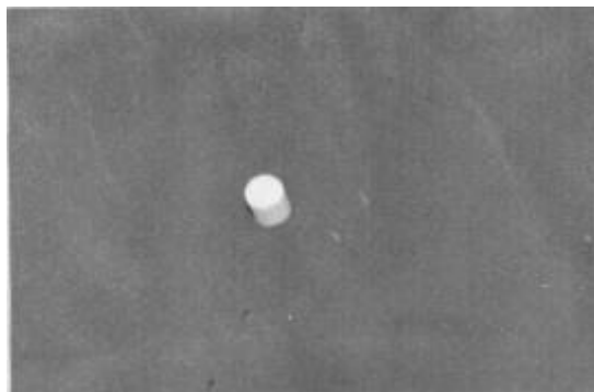
Figure 1. This is a cylindrical implant with 6.5mm in diameter and 5mm in height.
